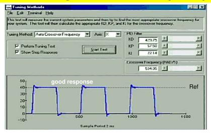
SDK applies driving signal to the motor and watching over the response of the motor the system parameters and best 9 controller parameters are determined.
