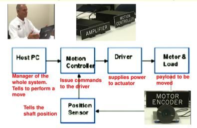
Closed loop motion control systems ⇒ Servo systems Some motion control systems are open loop (step motor systems) - There's no feedback loop, no tuning involved <sup>3</sup>
