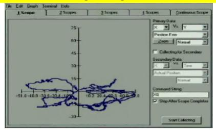
PID filter is tuned to shrink the error envelop as small as possible. Tuning PID filter: Start with initial PID gains, watch the error, change the gains, repeat motion, obtain error envelop, calculate the change of error, $_{17}$  update gains ...
