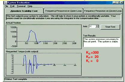
Deliberately introduce A MAJOR DISTURBANCE, which saturates the amplifier, and check and make sure that the position is still stable.
